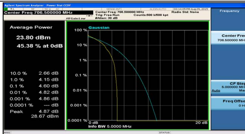
(Channel Bandwidth: 5 MHz)_LCH_QPSK_1RB#24
