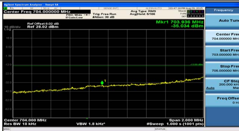
(Channel Bandwidth: 5 MHz)_LCH_16QAM_12RB#13
