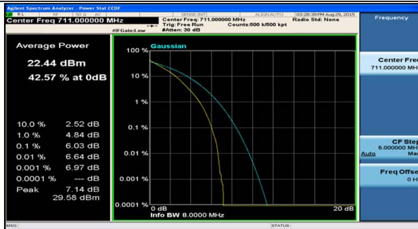
Channel Bandwidth: 10 MHz_HCH_QPSK_25RB#25
