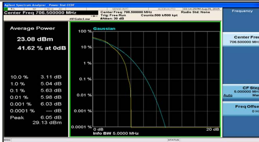
(Channel Bandwidth: 5 MHz)_LCH_16QAM_1RB#12
