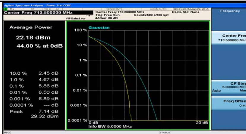
(Channel Bandwidth: 5 MHz)_HCH_QPSK_25RB#0
