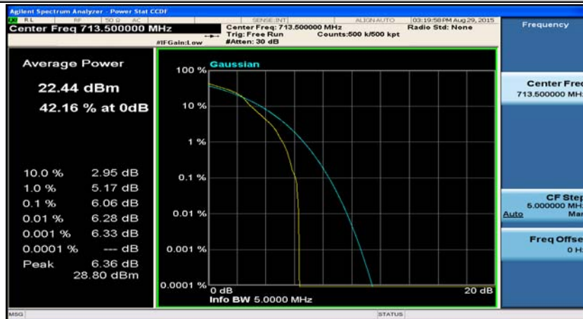
(Channel Bandwidth: 5 MHz)_HCH_16QAM_1RB#24
