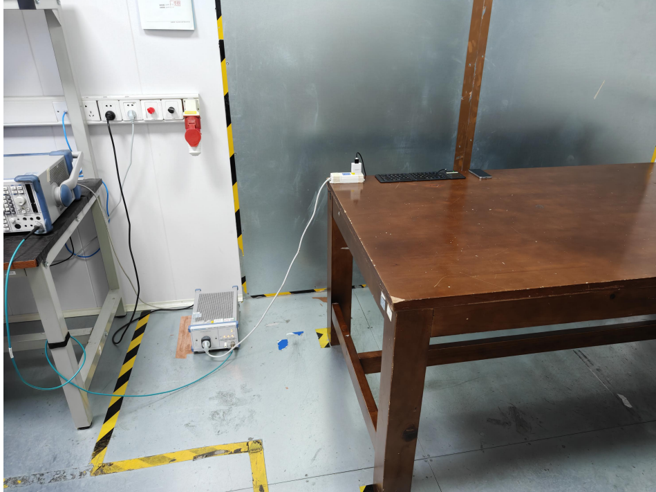
Conducted emissions at AC power line (150kHz-30MHz)
