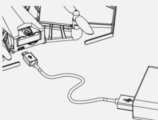
2.2 Plug batteries into the charger till they are buckled together. (Note: the charger is not included in the standard package and needs to be bought additionally.)
