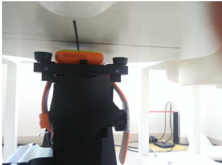
Face-held, the front of the EUT towards phantom (The distance was 10mm)
