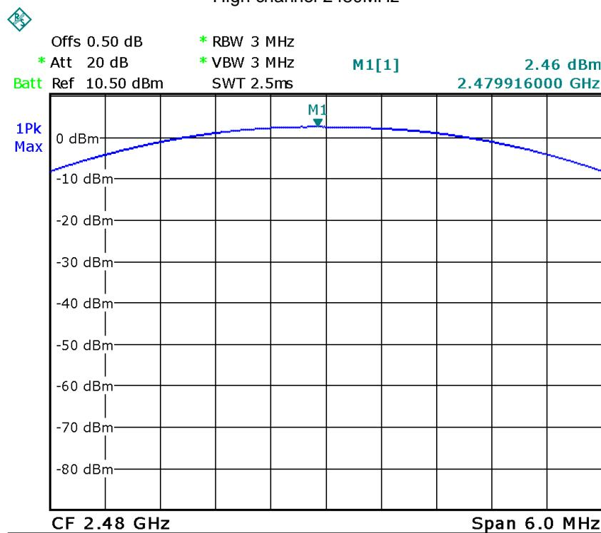
Bluetooth Mode  $\pi/4$ -DQPSK modulation Test Result
