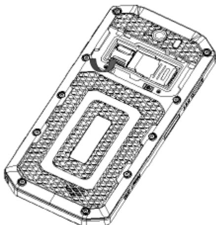
5.Insert the battery cover: Insert the back cover and rotate two screws clockwise to lock the back cover.
