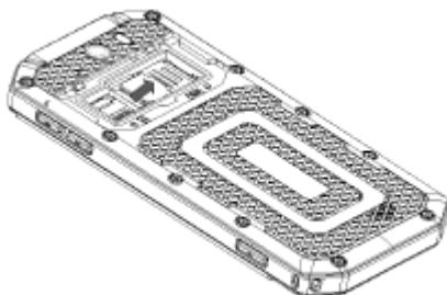
Note: When inserting the SIM card, ensure that the golden contacts faces right position.
