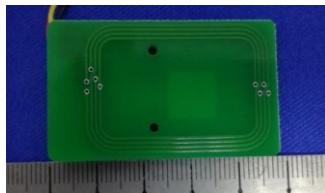
The antenna is a loop antenna and no consideration of replacement.
