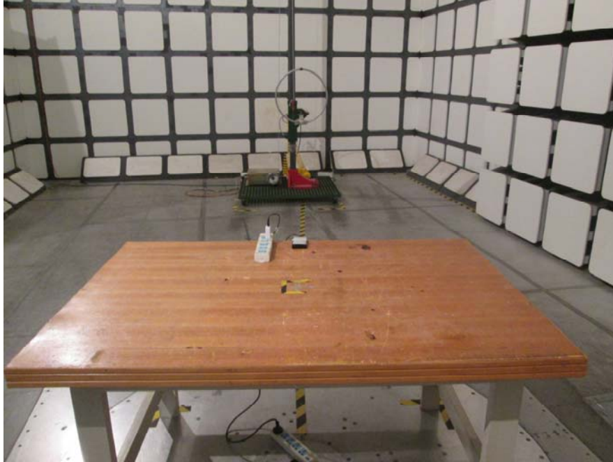
Radiated Emissions – Front View (Below 30 MHz)
