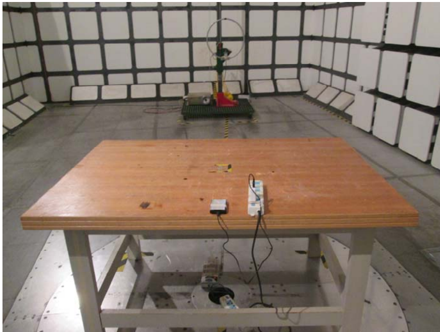
Radiated Emissions – Rear View (Below 30 MHz)
