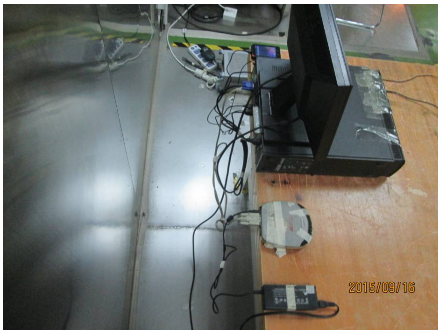
Conducted Emissions - Side View
