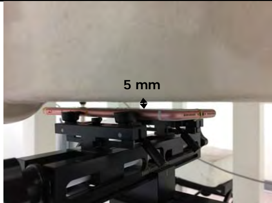
Fig.7 EUT Front side to flat phantom (No Case)
