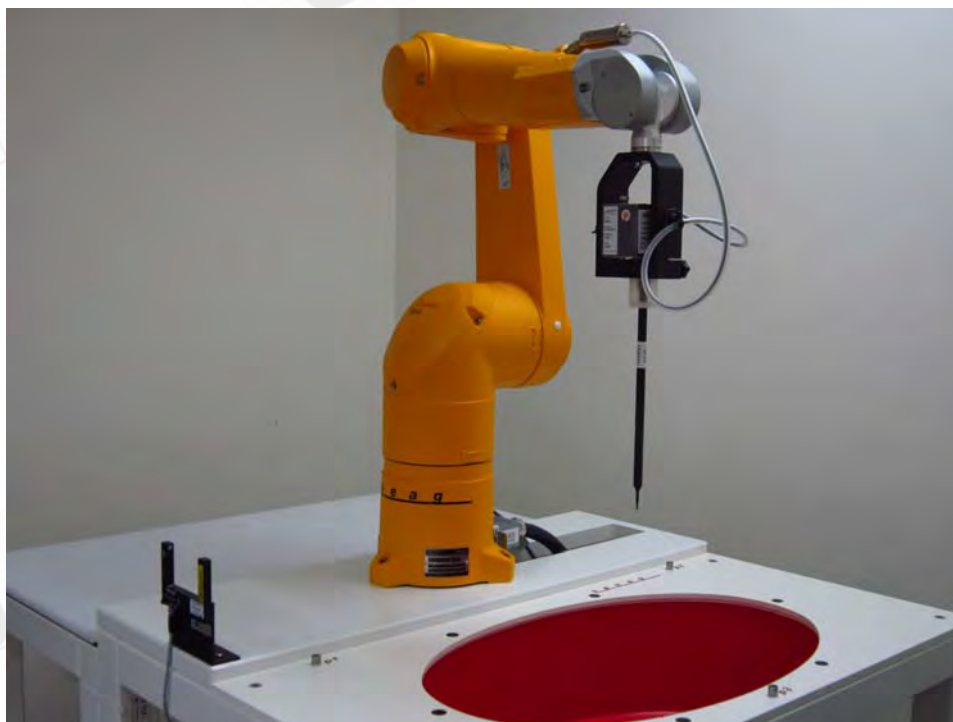
Fig.1 Photograph of the SAR measurement system
