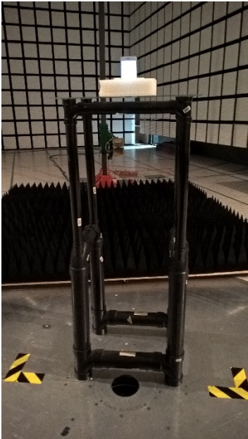
Figure 3.6-3: Setup photo – Radiated Emissions above 1GHz
