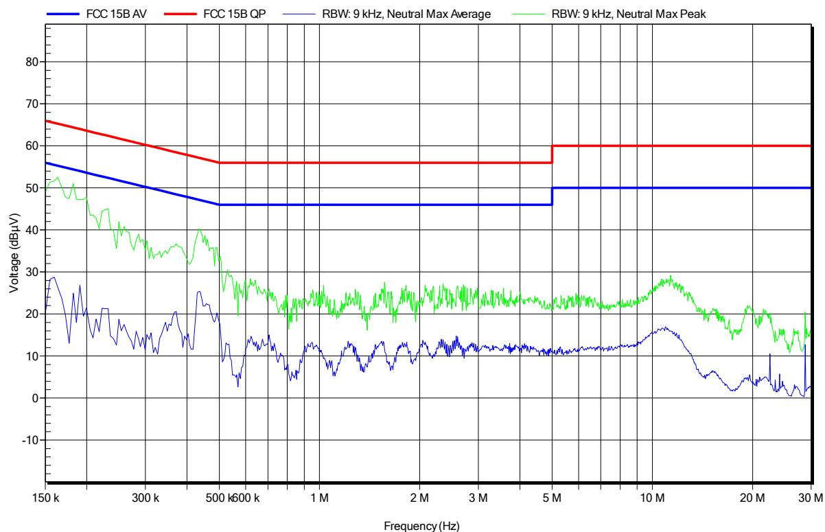
**EMI voltage test in the ac-mains according to FCC 15B**
