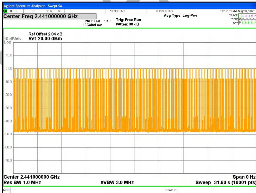
Dwell NVNT 1-DH3 2441MHz Ant1 One Burst
