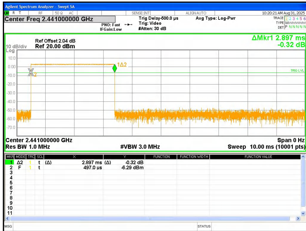
Dwell NVNT 1-DH5 2441MHz Ant1 Accumulated
