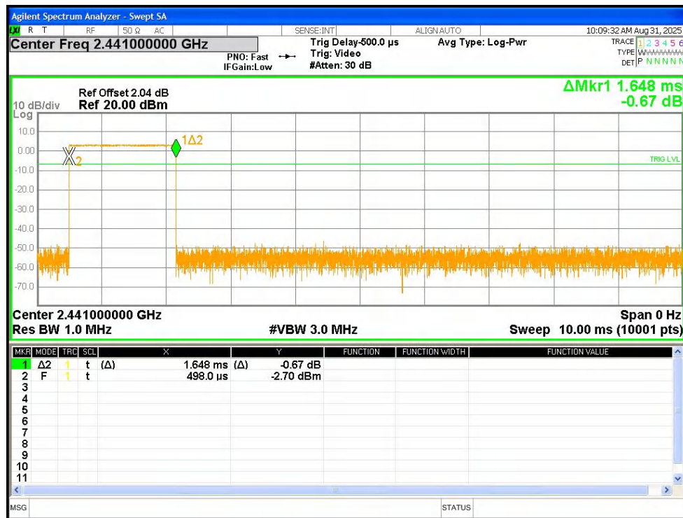
Dwell NVNT 1-DH3 2441MHz Ant1 Accumulated
