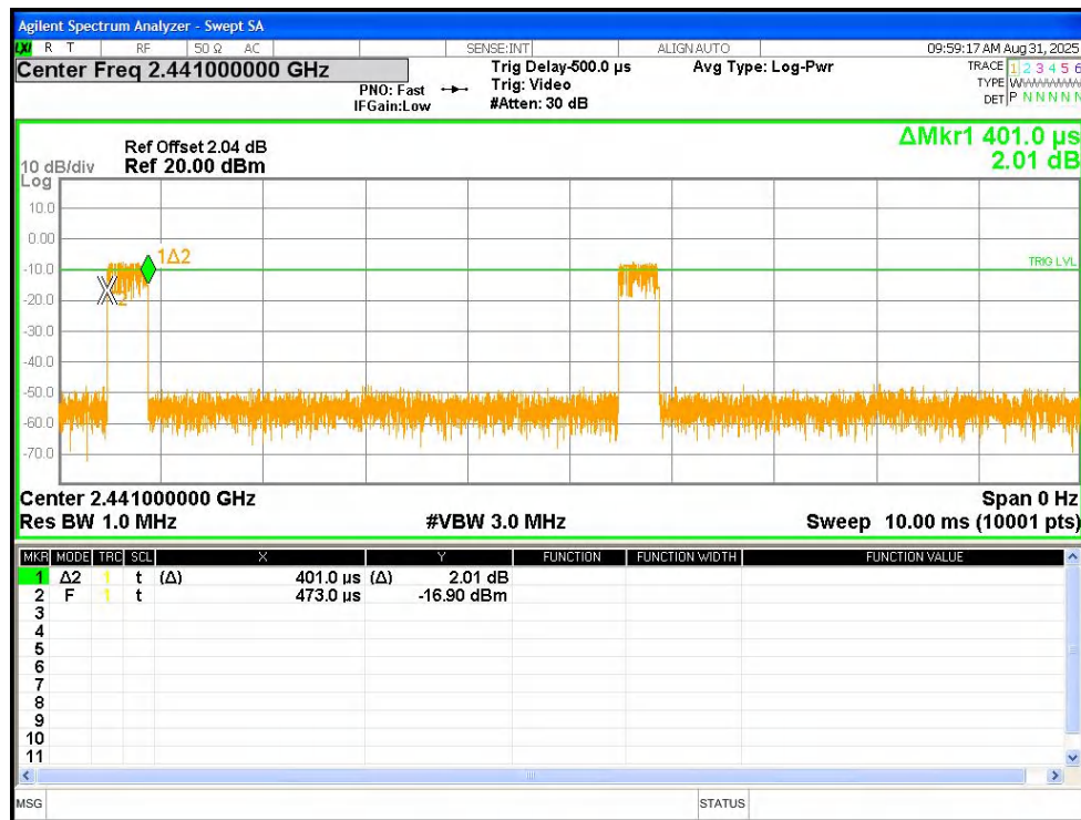
Dwell NVNT 3-DH1 2441MHz Ant1 Accumulated
