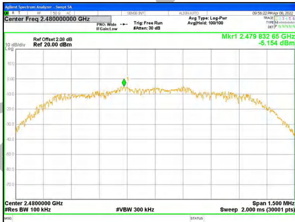
Tx. Spurious NVNT 3-DH1 2480MHz Ant1 Emission
