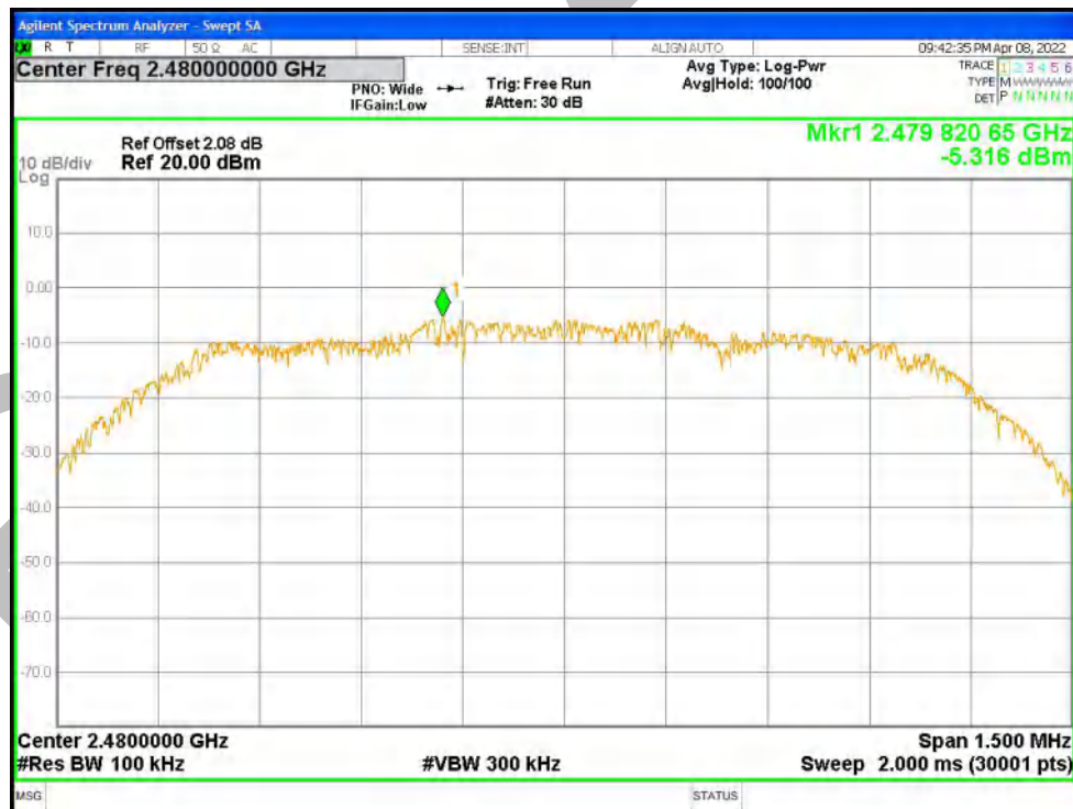
Tx. Spurious NVNT 2-DH1 2480MHz Ant1 Emission
