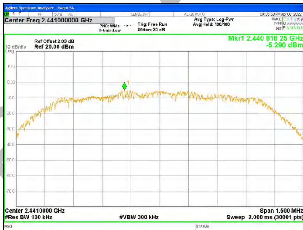
Tx. Spurious NVNT 2-DH1 2441MHz Ant1 Emission
