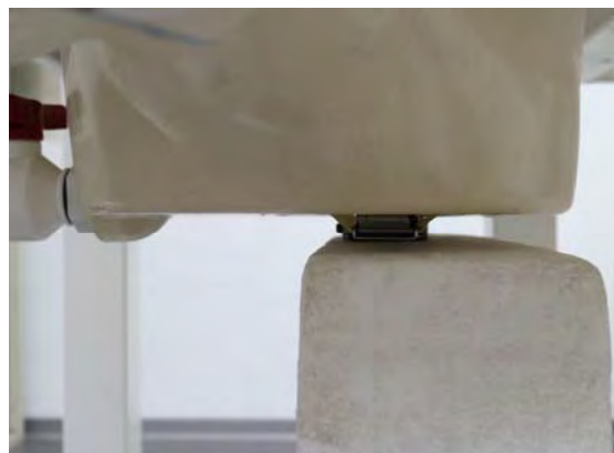
Fig.3 Configuration 1: watch's back touch against the flat phantom (gap: 1.25mm)
