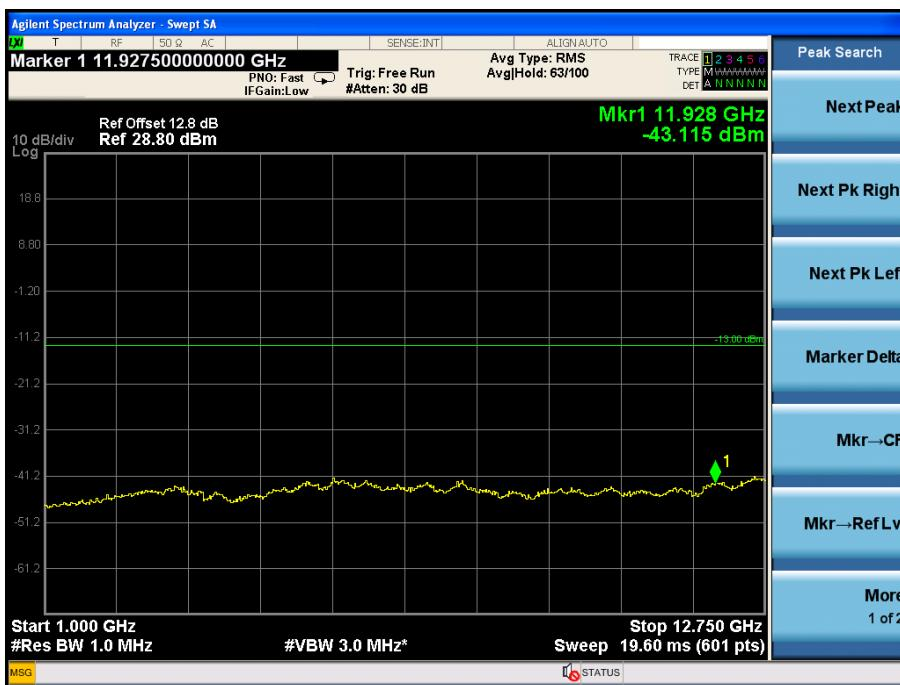
Test Mode: GSM 850 CH 251
