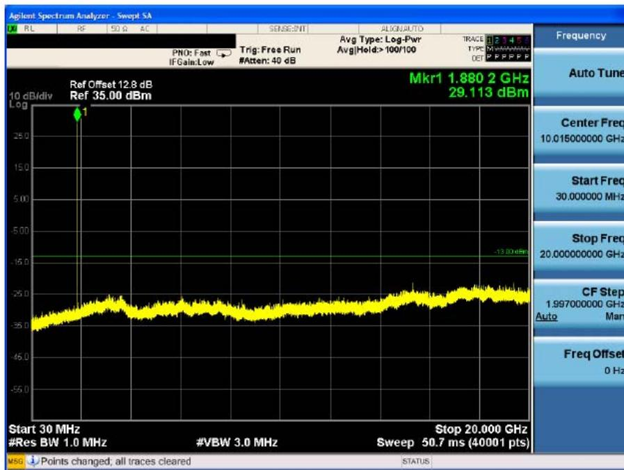
Test Mode: GSM 1900 CH 810
