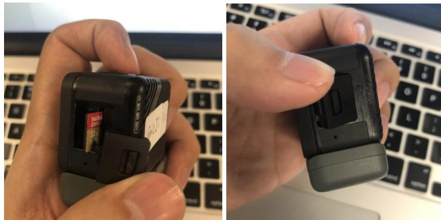
Press firmly on the cover, and make sure that the yellow color at the button is no longer displayed, it is considered to be completely covered with a waterproof board.
