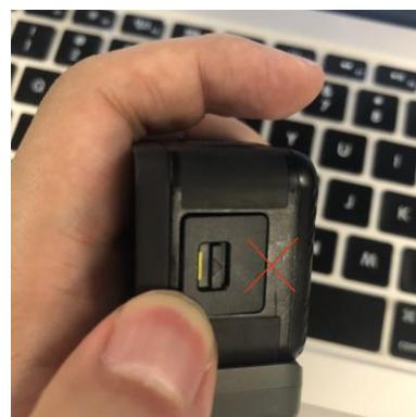
Please note that the button on the cover and the microphone hole on the bottom are in a vertical line for the correct orientation. If installed in the opposite direction, there may be a risk during exercise. The camera
