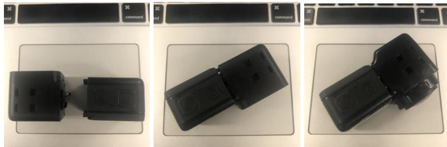
Once the lens and body are installed, align them with the metal slots of the battery and press firmly to ensure that the battery clips completely catch the lens and body.
