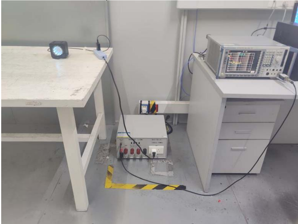
Photos of power line conducted emission test
