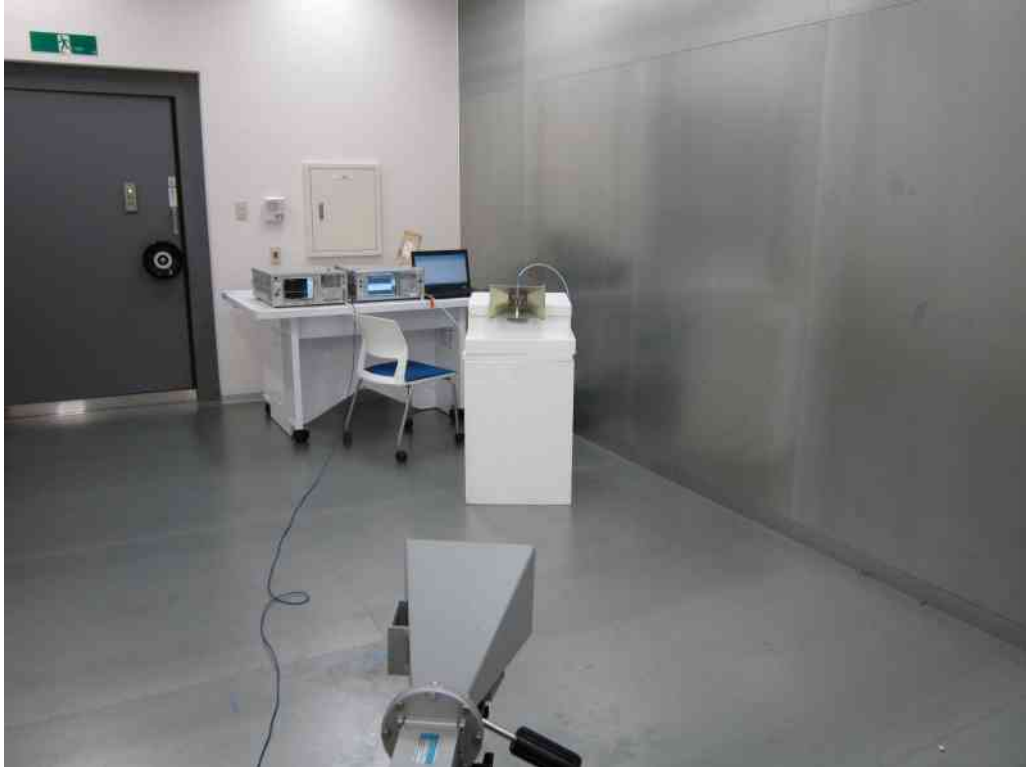
Test Setup for Generating the Radar Waveform
