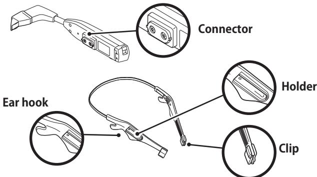
1. Slide the device connector to insert it into the neckband holder.
