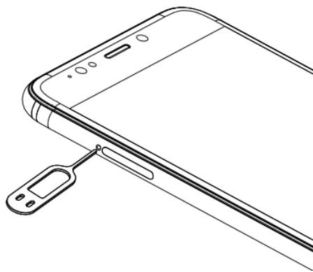
2) Put Nano SIM cards and SD card to card tray correctly.
