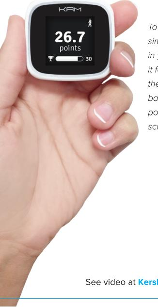
To change screens, simply hold the KAM in your hand and tilt it forward towards the ground. Tilt it back up again to this position. The next screen will appear.
