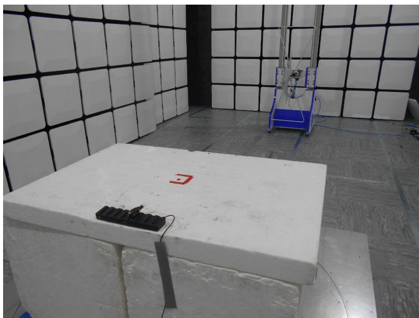
Photo 2.3-2 – RE Spurious Emissions 30-1000 MHz – Back Side
