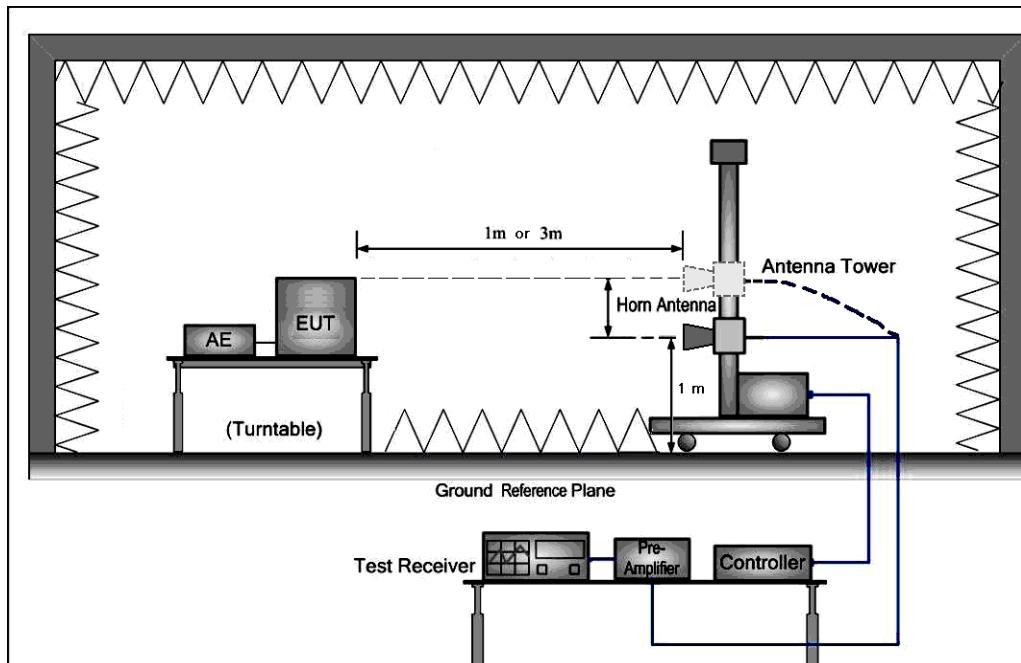
The field strength is calculated by adding the Antenna Factor, Cable Loss & Per-amplifier. The basic equation with a sample calculation is as follows:
