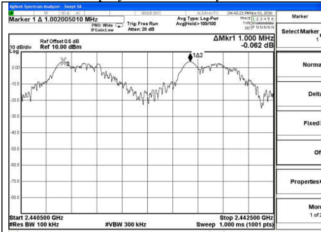
Test Plot Of Frequency Separation (1Mbps)
