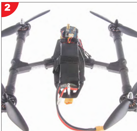
2 Installation the full charged flight battery into the CROSSFIRE.
