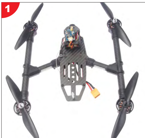
1 Installed the four rotors in properly.
