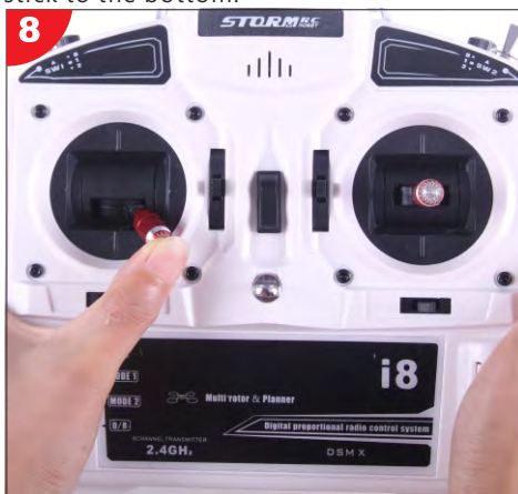
8 ARM the main flight controller system
