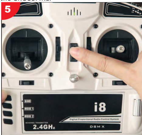
5 Power on the transmitter, and put the throttle stick to the bottom.
