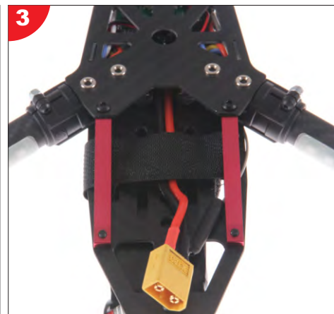
2 Installation the full charged flight battery into the CROSSFIRE.
