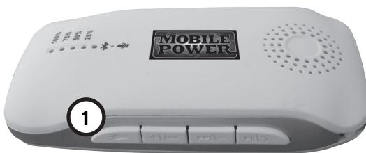
2. Connect USB portable device into the unit's USB port using the Power Bank Micro USB cable provided or charging cable provided with USB device. *Note: If a device is not connected to the Power Bank USB port within 20 Seconds of activating the USB port; it will turn OFF automatically and it will require to press the Light Button once again to activate it.*
