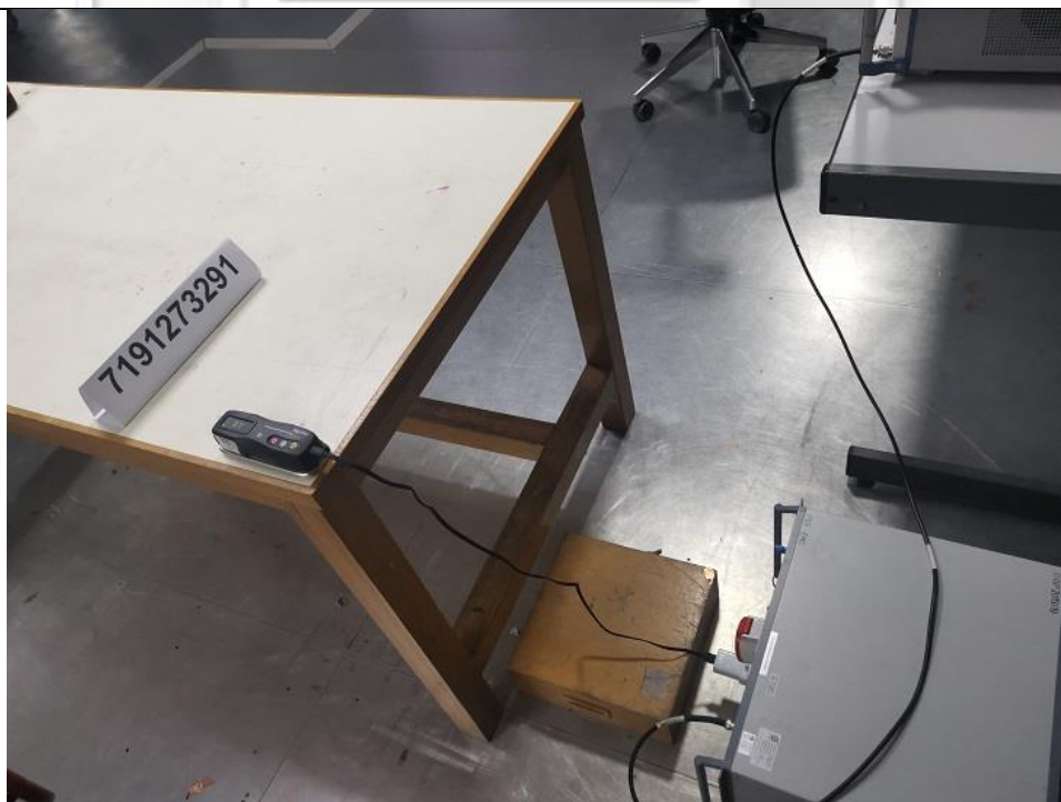
Conducted Emissions Test Setup (Rear View)
