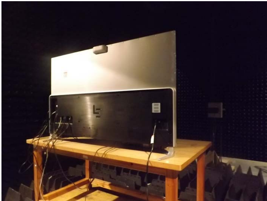
Photograph - Conducted Emissions Test Setup
