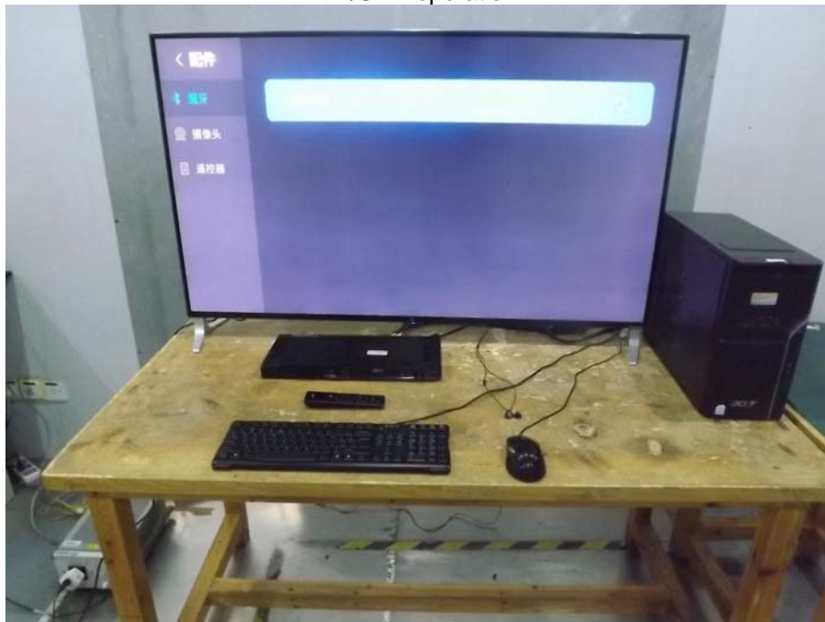
Photograph - Conducted Emissions Test Setup
