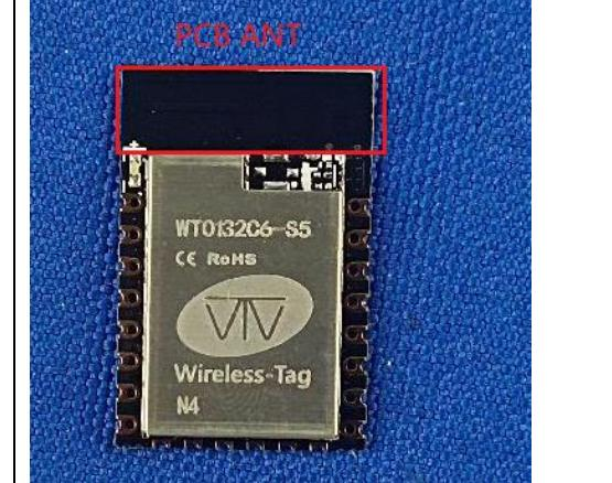
A photograph of the WT0132C6-S5 module. It is a square PCB with a single black PCB antenna on top. A red box highlights the PCB ANT. The module is mounted on a blue fabric surface.                                                               |
