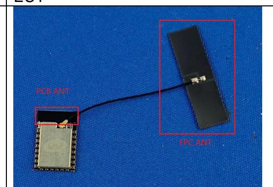
A photograph of the WT0132C6-S5U module. It is a square PCB with a small black PCB antenna on top and a larger black FPC antenna attached by a cable. Red boxes highlight the PCB ANT and FPC ANT. The module is mounted on a blue fabric surface. |
