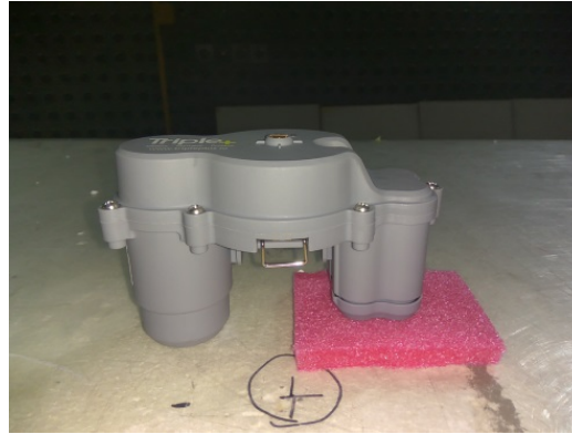
Photograph 6.4.2 EUT in Y-axis orthogonal position
