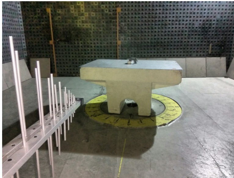
Photograph 8.1.1 Setup for radiated emission measurements
