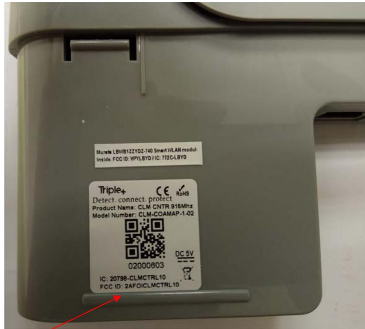
Label with **FCC ID:2AFOICLMCTRL10** and **IC:20798-CLMCTRL10** is located at the bottom side of the HUB. The statement according to FCC part 15 §15.19(a)(3) is placed in User's Manual, page 26 (Application exhibit User\_manual\_28549).
