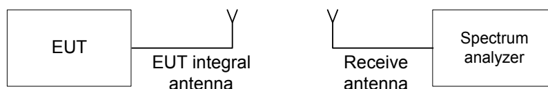
Figure 7.1.1 Setup for transmitter shut down test
