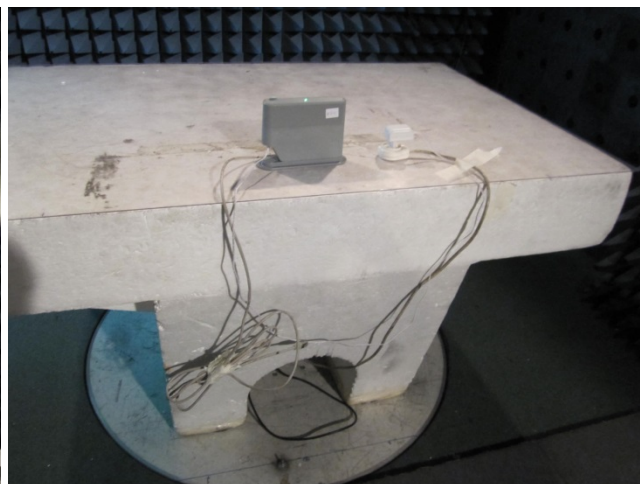
Photograph 8.2.1 Setup for radiated emission measurements
