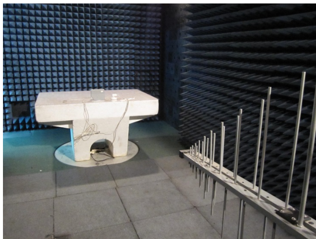
Photograph 8.2.1 Setup for radiated emission measurements
