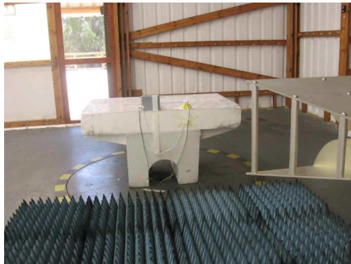
Photograph 8.2.2 Setup for radiated emission measurements, general view
