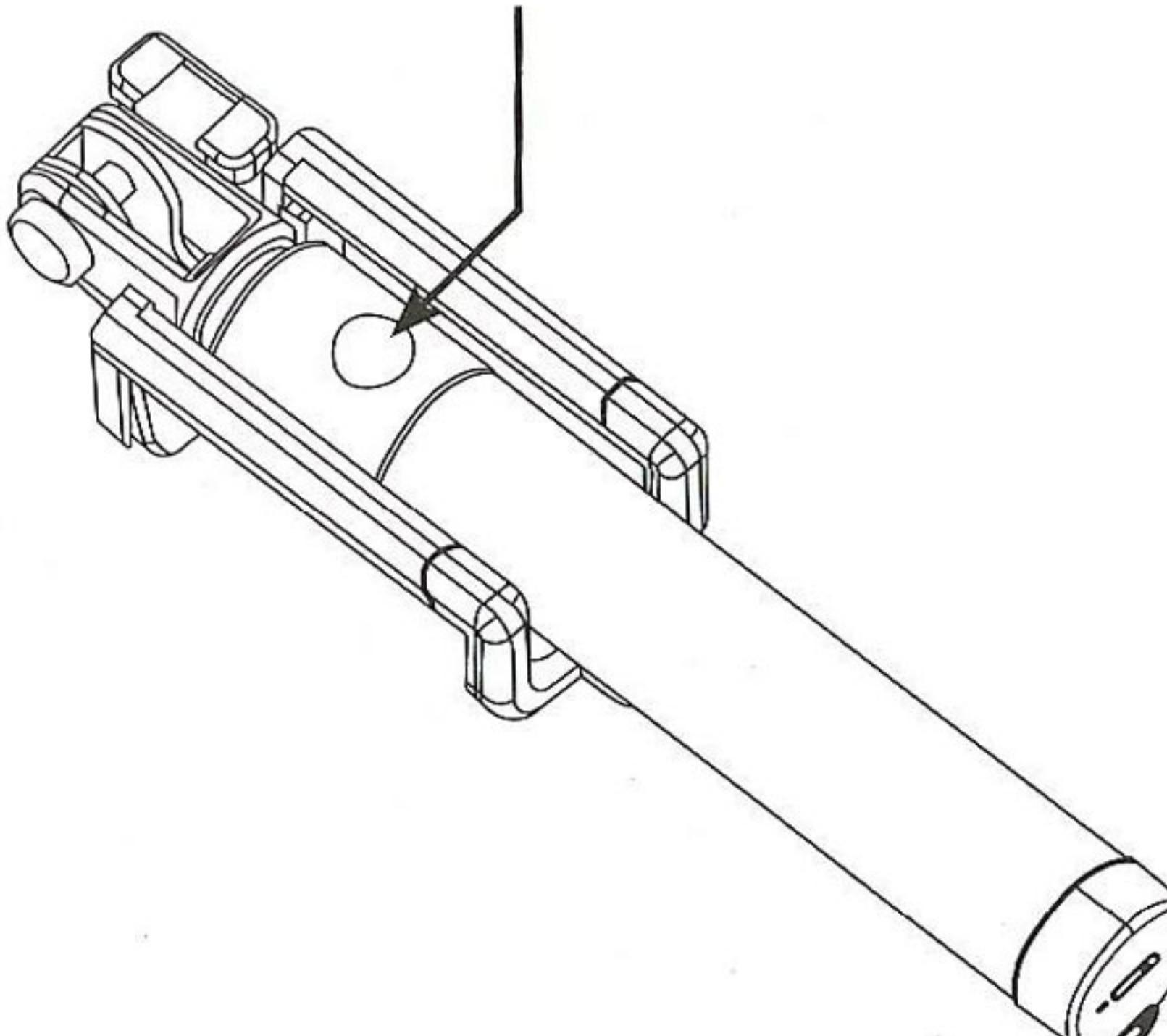
Long-press the key for 3s, the blue light will flash and the camera enters the Bluetooth pairing mode.
