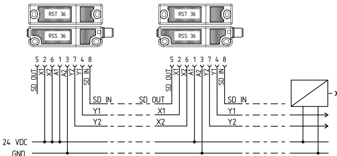
Y1 and Y2 = Safety outputs → Safety monitoring module
