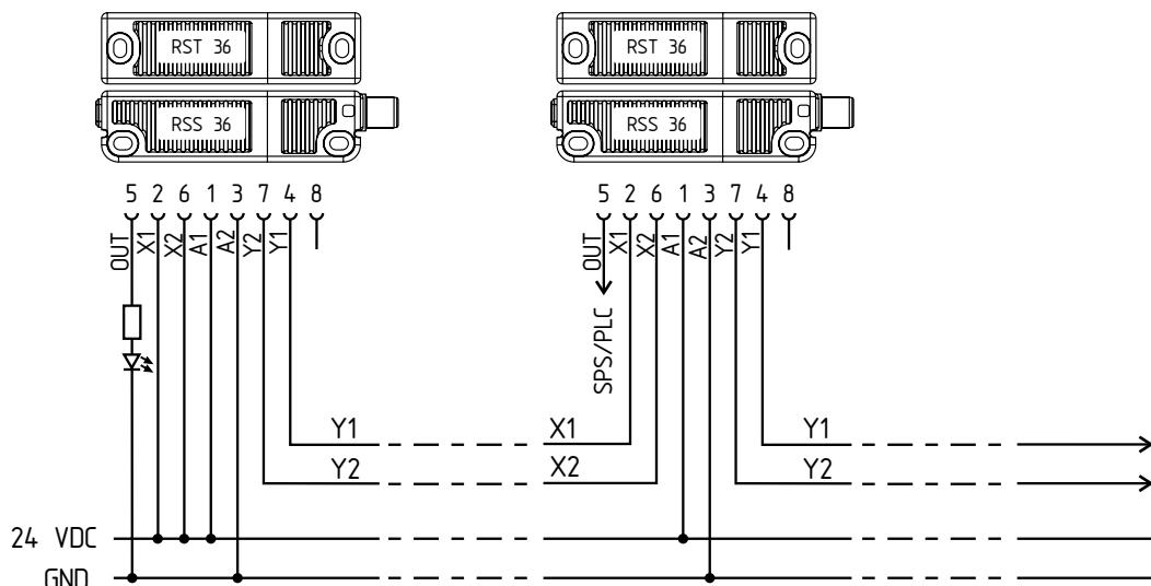
Y1 and Y2 = Safety outputs → Safety monitoring module
