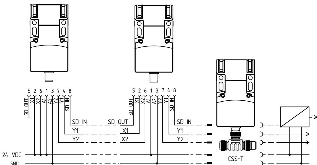
Y1 and Y2 = Safety outputs → dual-channel safety monitoring module
