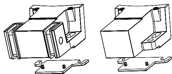
It is recommended to use the attached shims when using the securing slots or placing on a flat surface (not when actuating on the floor).
