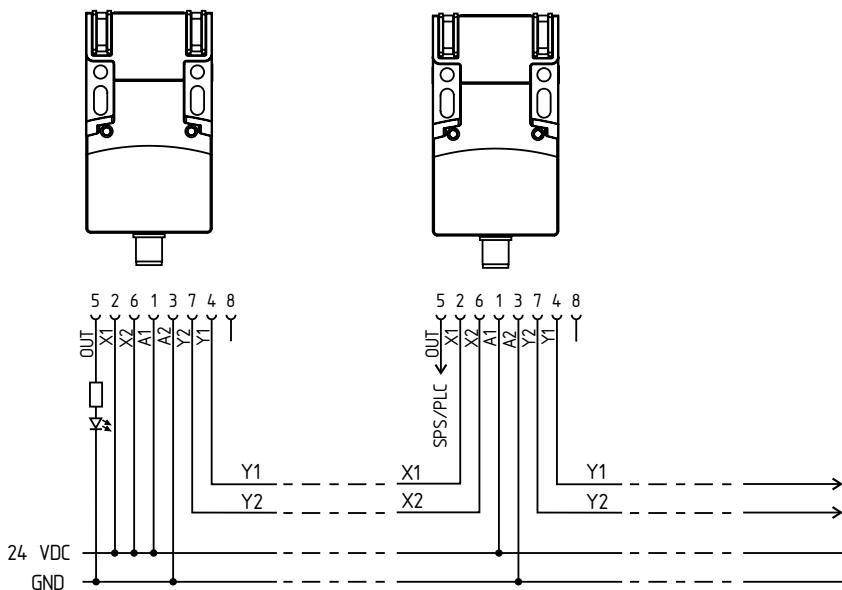
Y1 and Y2 = Safety outputs → dual-channel safety monitoring module
