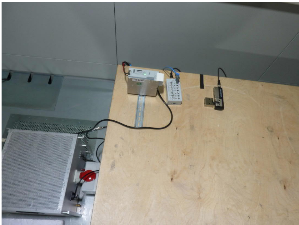
210165_02: Test setup conducted emission test 150 kHz – 30 MHz
