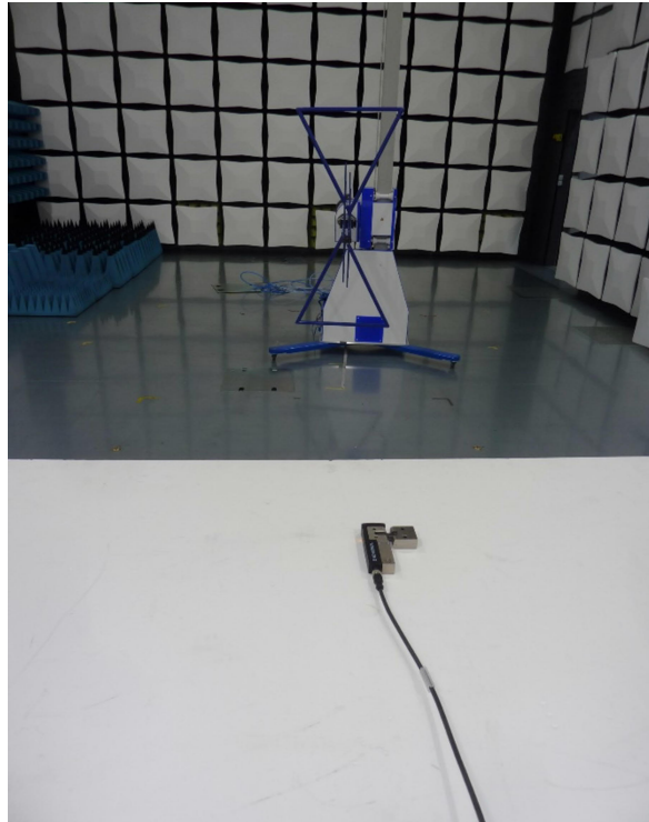
210165_05: Test setup radiated emission test 30 – 1000 MHz
