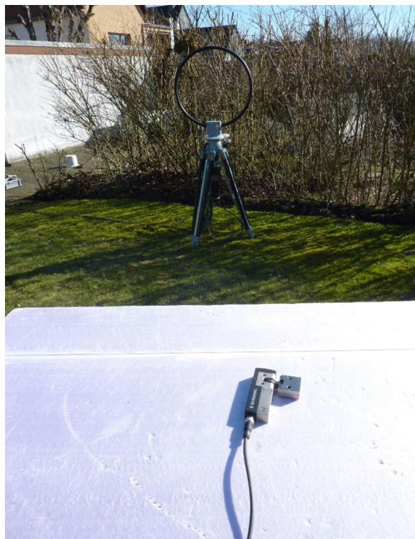
210165_04:Test setup final radiated emission test 150 kHz – 30 MHz
