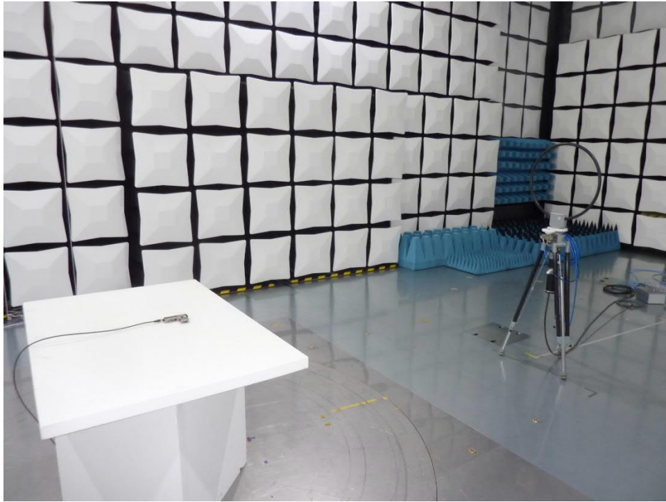
210165_03:Test setup preliminary radiated emission test 150 kHz – 30 MHz
