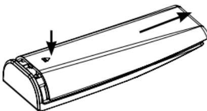
2. Insert the batteries, paying attention to match up the (+) and (-) ends of the batteries with the symbols inside the battery compartment.
