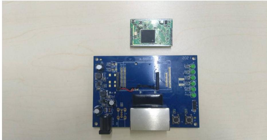
**Step 2:** put the module module to ensure that: (1) Make sure that the module antenna near the baseplate edge (2) the needle of the module should be one-to-one correspondence with bottom row of socket pair as shown in figure
