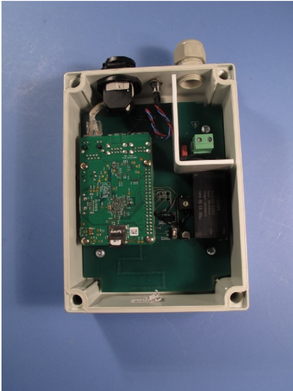
Photograph 1: Internal view of Concentrator
