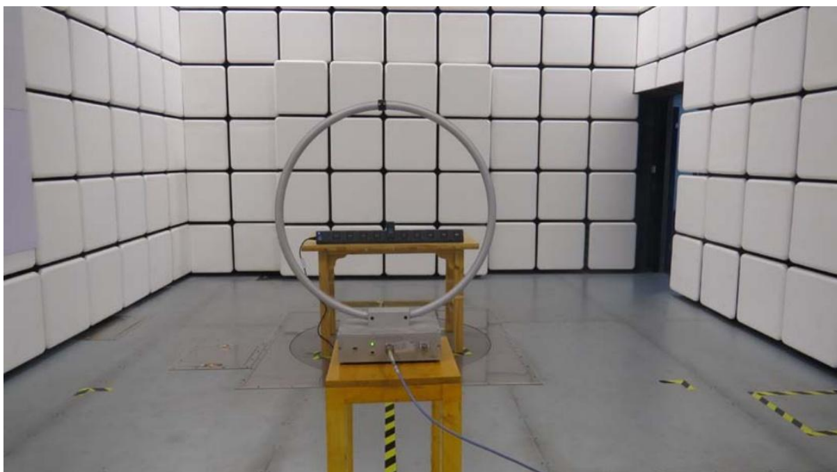
Radiated Emission Test Setup 9 kHz – 30 MHz
