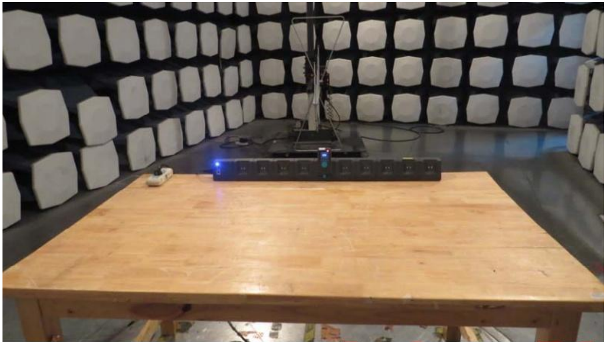
Radiated Emission Test Setup 30 MHz – 1 GHz
