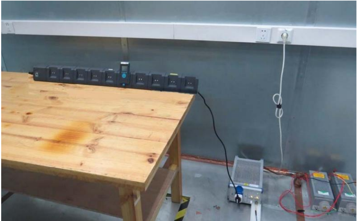
Conducted Emission Test Setup
