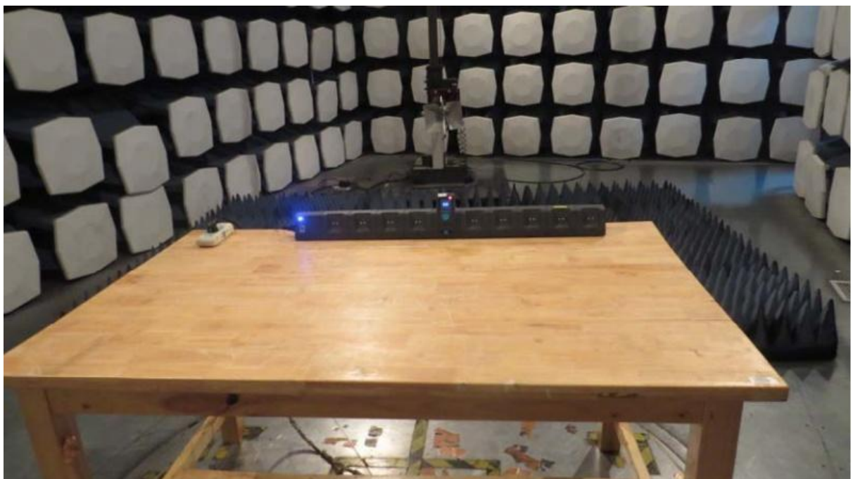
Radiated Emission Test Setup – Above 1 GHz
