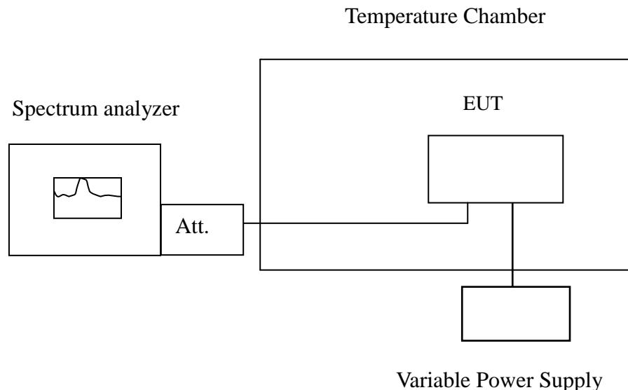
**Remark:** Measurement setup for testing on Antenna connector
