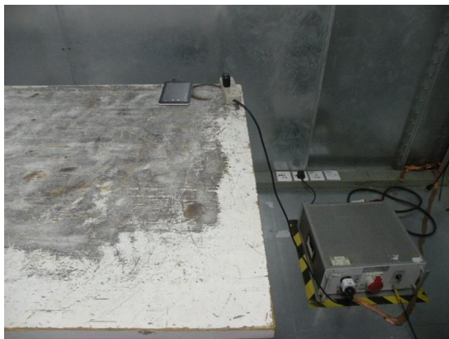
Photos of Conducted Emission test
