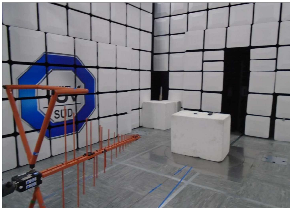
Figure 19 - Test Setup - 30 MHz to 1 GHz
