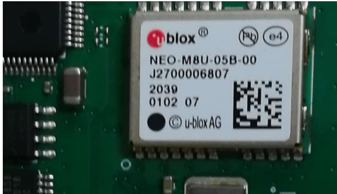
Figure 4: Close up view of GNSS
