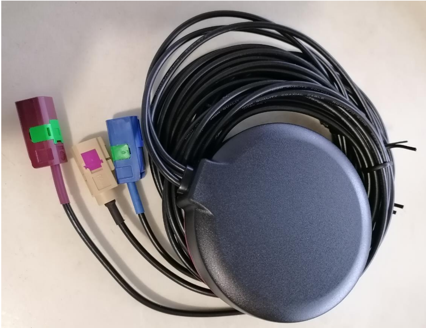
Figure 7: PUCK Antenna: LTE Diversity (purple), WiFi/BT (beige) and GNSS (blue)
