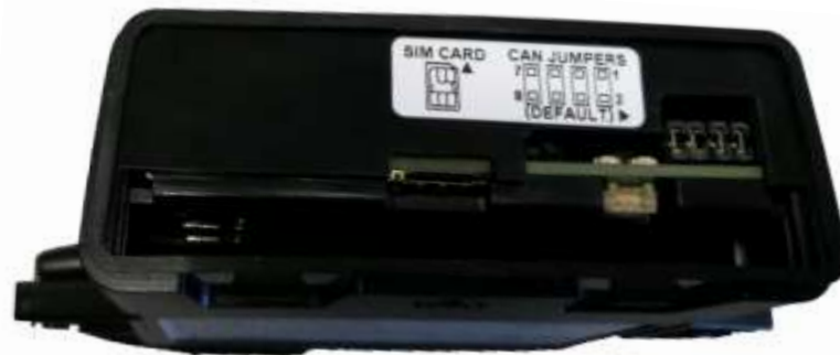
Figure 7: Position of jumpers on the PCB.
