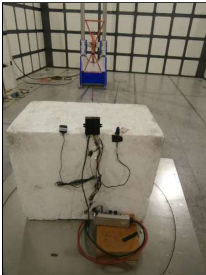
Figure 28 – Test Setup – 30 MHz to 1 GHz, Y Orientation
