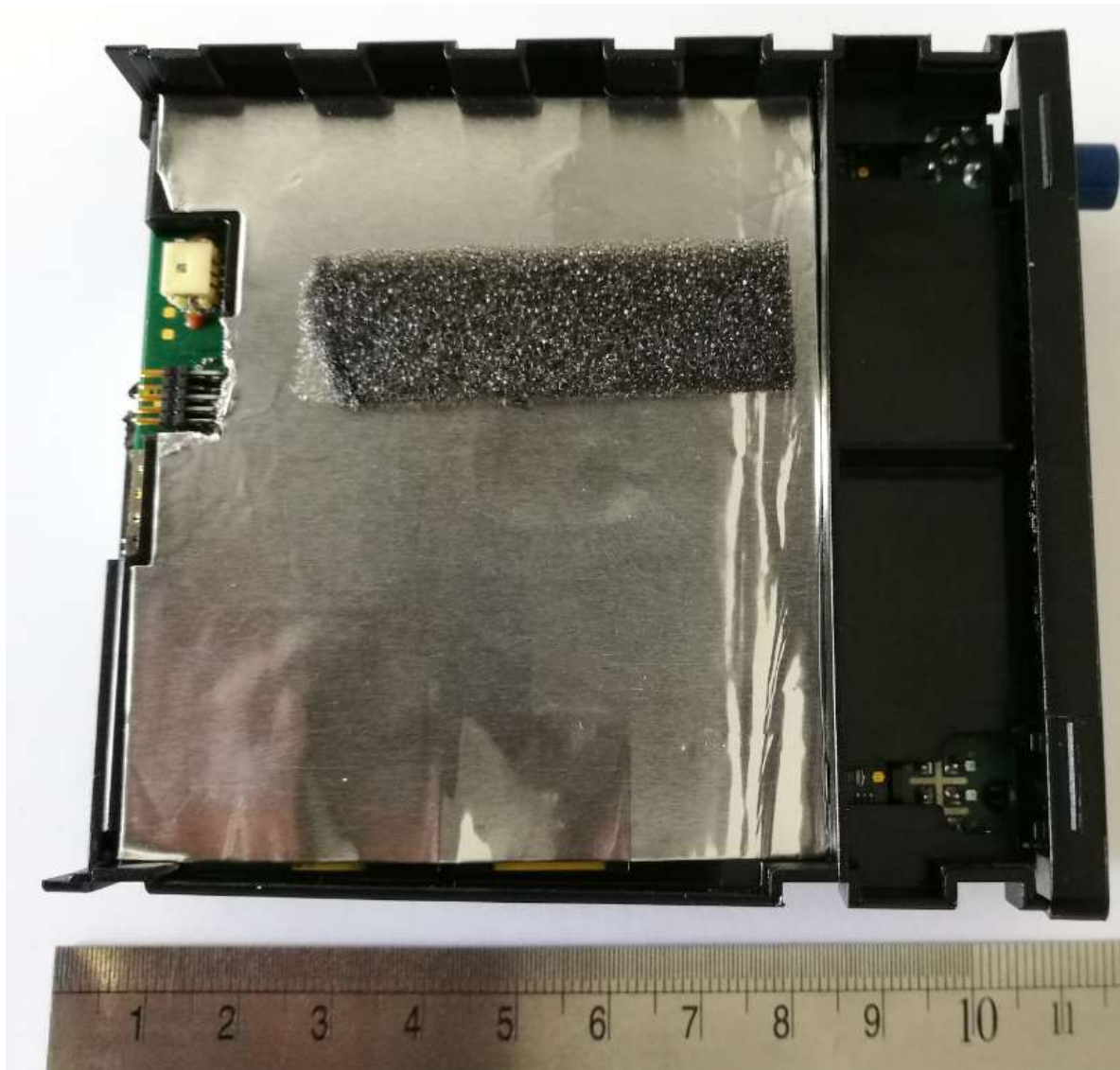
Figure 6: Bottom Side of Main PCB on Carrier – battery NOT fitted (MiX 44MC-3G)
