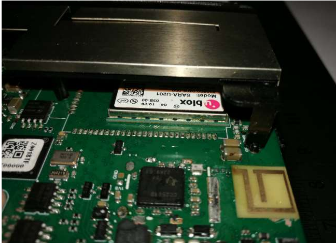
Figure 5: View of Main PCB – Modem and Bluetooth without shield
