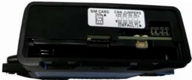
Figure 7: Position of jumpers on the PCB.
